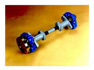
The Layrub range is a long established but still unique design based on a range of twelve standard blocks. It is generally used to cover the low to medium power ranges up to torque ratings of 64 kNm. The blocks can be used in parallel leading to compactness and making the coupling suitable for high speed operation or in series to provide a torsionally soft coupling and to accommodate large mis-alignments.
