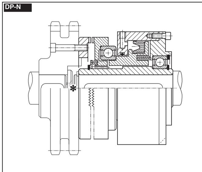
**TOOTH-TYPE PNEUMATIC COUPLING SPRING LOADED**
