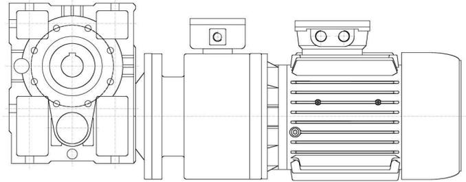
*Standard B5 motor + VIS brake + gearbox unit*
