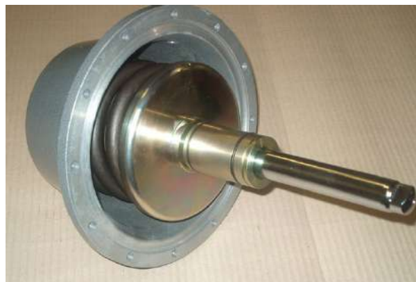
FIGURE 14 – Centre Casing removed (rear diaphragm removed)
