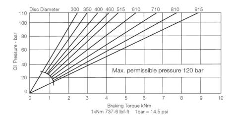
Brake Perfomance of T20 Disc Brake Caliper
