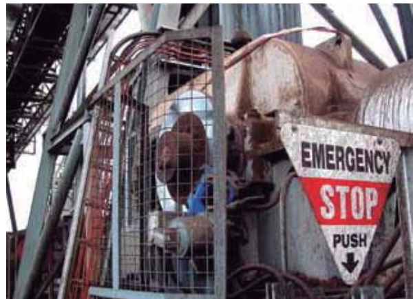
Twiflex GMR-SH spring-applied hydraulic released brake units fitted to a power station conveyor in Victoria, Australia.
